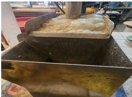
Figure 1. Denver flotation cell at Peacock and Simpson Laboratory. The cell was used for all rougher flotation experiments in this study, operated at 1200 rpm impeller speed and 6 L/min air flow rate. The trough and scraper arrangement shown are consistent with the Denver D-12 laboratory flotation unit used for batch rougher flotation tests on 1 kg ore charges.
